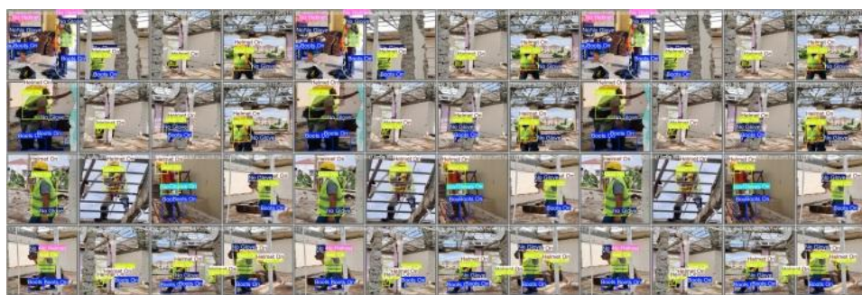
Figure 5. Example of Visual Detection Results (Bounding Box) from YOLOv8, YOLOv11, and YOLOv12 original image, saturation level 30%, and -30%
