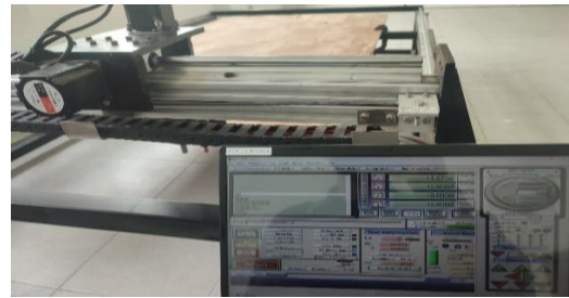
Figure 19. Position of the X-axis after receiving a pulse input command via the CNC controller.
