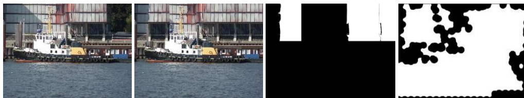
Figure 12 From left to right : Original image, multiple copy-move image, ground truth, result map of the detection.
