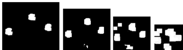
Figure 15 Effect in Gaussian Pyramid in detection result in different size (in pixels); Left to right : 512 \times 512 , 256 \times 256 , 128 \times 128 and 64 \times 64 (Shabanian & Mashhadi, 2018)
